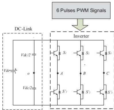
Gambar 1. Skema sistem inverter dua-level tiga-fase
