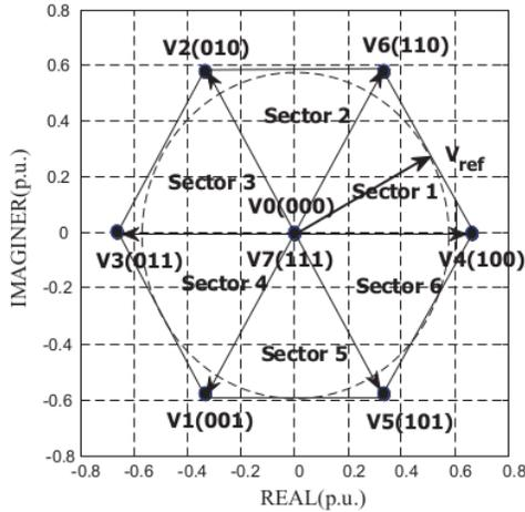
Gambar 4. Tegangan space vector inverter dua-level tiga-fase
