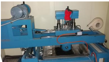
Loading wheel track
