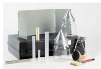
Alat uji sand patch
