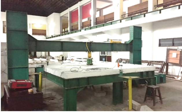
Fig. 3. Slab test set-up.
