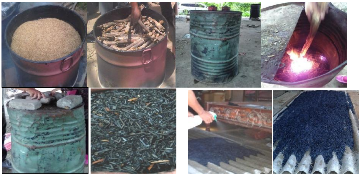
Figure 1. Biochars process from agricultural waste (fresh rice husk and wood)
