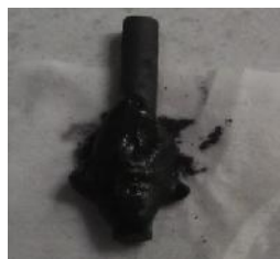
Figure 2. Put electrolyte and positive electrode (graphite) on separator (tissue)
