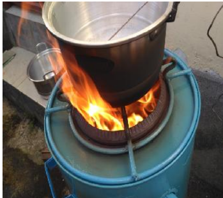
Figures 8 Visual condition of the flame generated by the designed stove no 5
