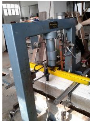
Figure 5. Flexural test using Wykeham Farrance Machine
