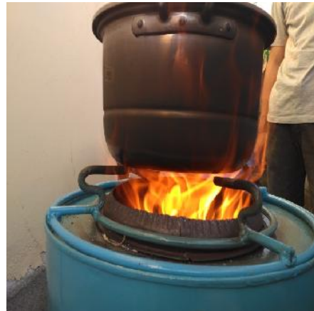
Figures 9 Visual condition of the flame generated by the designed stove no 6
