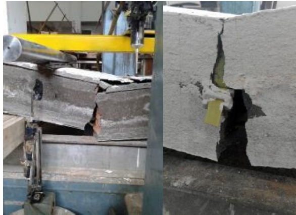
Figure 10. Specimen that cracked but did not fall apart
