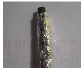
Figure 2. Put electrolyte and positive electrode (graphite) on separator (tissue)
