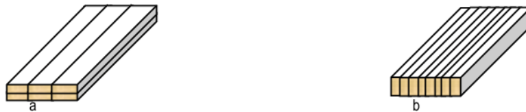
Figure 1. a) Strip arrangement the thick direction; b) Strip arrangement in the width direction.
