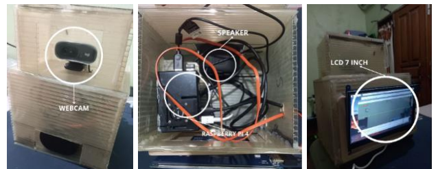
Gambar 9. Raspberry Pi 4, LCD, webcam , dan speaker .
