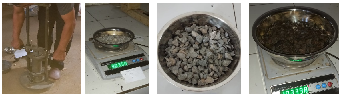
Impact test Water absorption Density Figure 4. Sample testing for impact value, water absorption, and density
