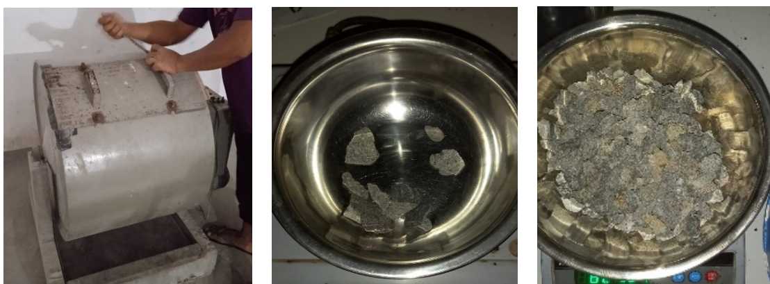
Abration test Aggregates shape Soundness test Figure 6. Sample testing for abrasion value, aggregates shape and soundness
