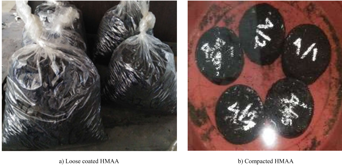
Figure 7. Asbuton mixture and specimens in the curing process
