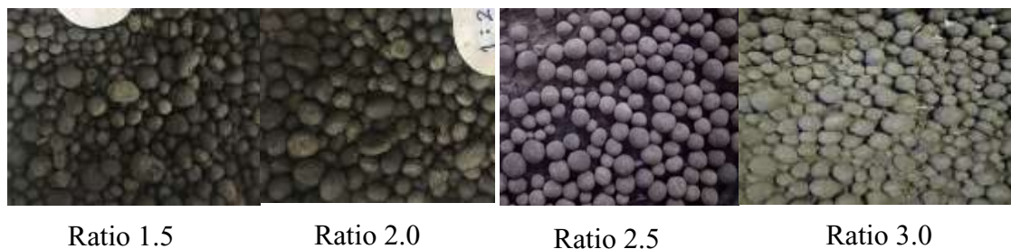
Fig 7. Artificial aggregates with a slope of 50^\circ and variations in the ratios of \text{Na}_2\text{SiO}_3/\text{NaOH}
