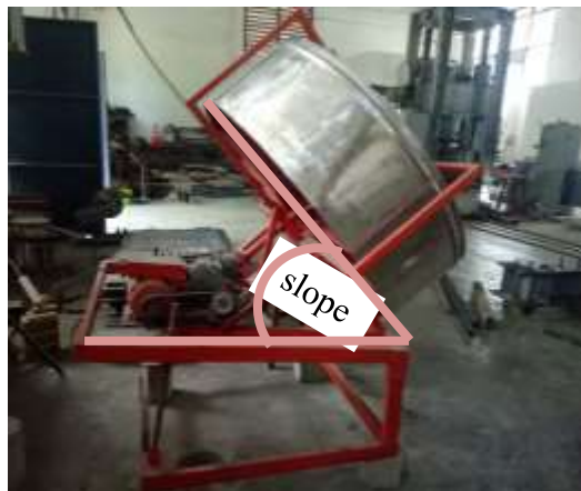
Fig 2. Granulator and pan slope
