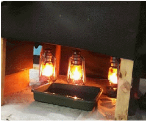
Photo 1. Kerosene mini stove for heating the sawdust
