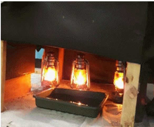
Photo 1. Kerosene mini stove for heating the sawdust
