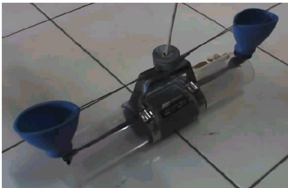
Gambar 4. Alat Ukur Water Sampler (LaMOTTE Model JT-1)
