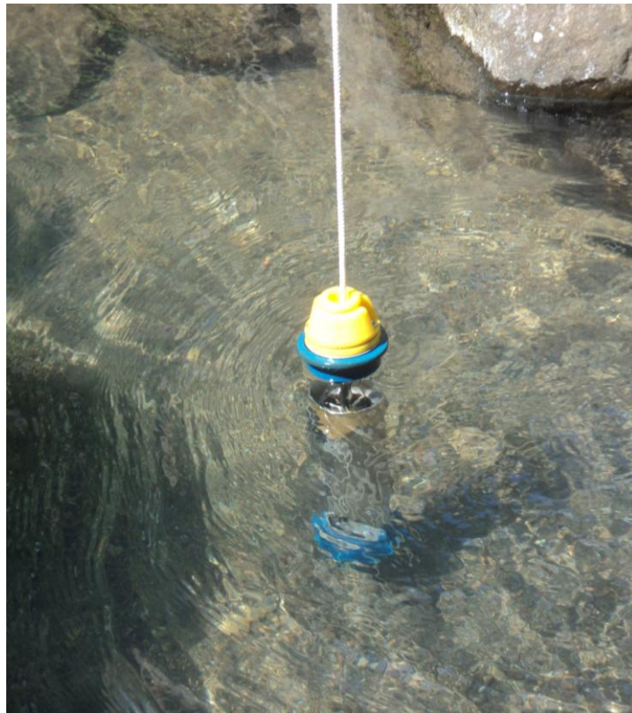
Gambar 12. Alat ukur water sampler vertikal
