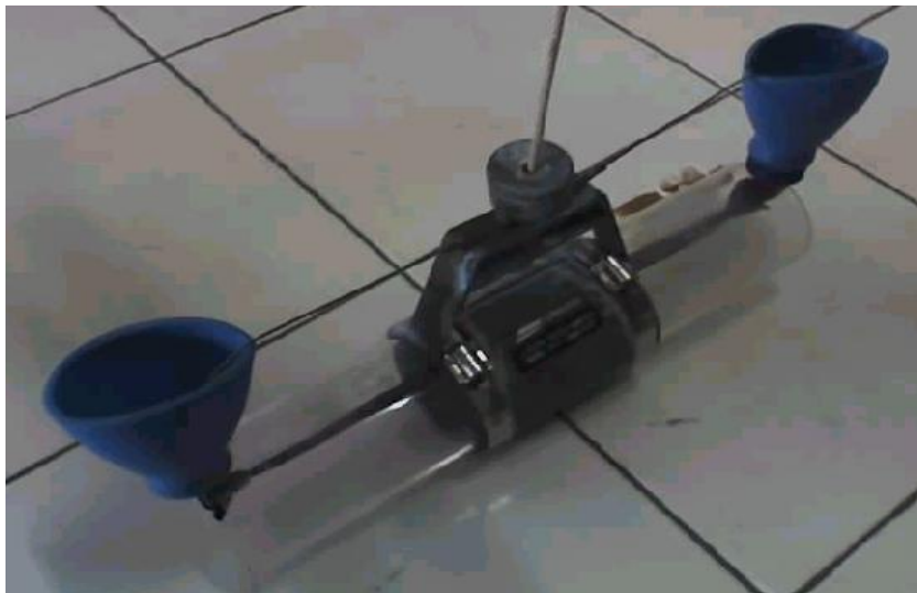
Gambar 4. Alat Ukur Water Sampler (LaMOTTE Model JT-1)
