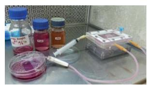
Figure 7. Parallel plate flow chamber built in the recent study used permeable membrane for growing cells, also used pediatric infusion set to get a small fluid capacity as low as 1ml/minute
