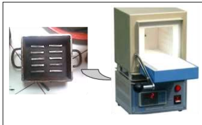
Figure.2. Pack carburizing process
