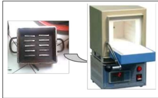
Figure.2. Pack carburizing process
