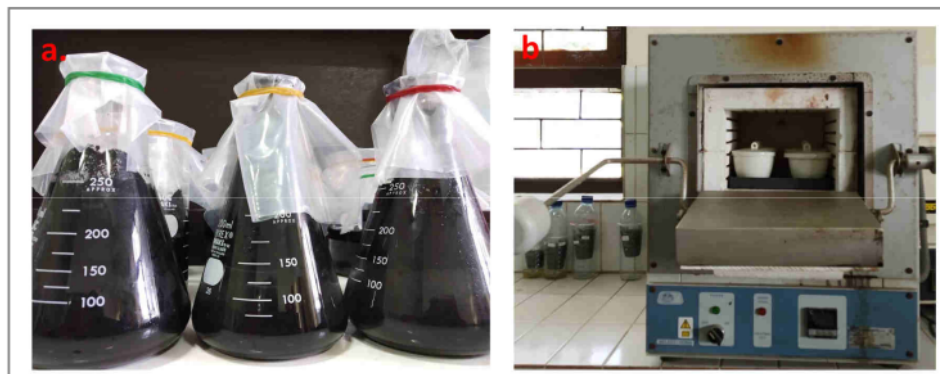
Gambar 2. Proses aktivasi secara kimia (a) dan fisika menggunakan furnace (b) Figure 2. Activation processes chemically (a) and physically using furnace (b)
