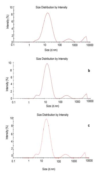
Figure 3. Particle size distribution powders generated from (a) chitosan (0.5% w/v) + maltodextrin (9.5% w/v) in acetic acid, (b) only
