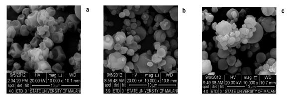
Figure 2. SME (10,000X) of spray-dried powders (a) chitosan (0.5% w/v) + maltodextrin (9.5% w/v) in acetic acid, (b) only maltodextrin (10% w/v) in liquid smoke, and (c) chitosan (1.5% w/v) + maltodextrin (8.5% w/v) in liquid smoke
