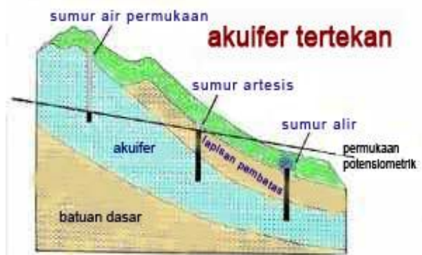
Gambar 2.3 Akuifer tertekan ( Confined Aquifer ) (Wuryantoro, 2007)
