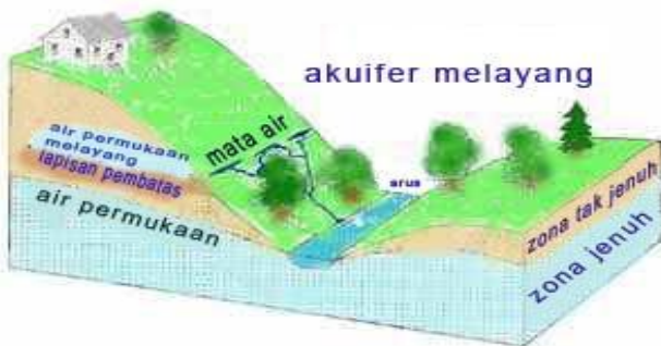
Gambar 2.4 Akuifer melayang ( Perched Aquifer ) (Wuryantoro, 2007)
